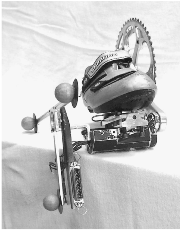
Fig. 2 Photograph of six-load-component pedal dynamometer with inversion/eversion interface attached. The interface also has a medial/lateral translational adjustment.
